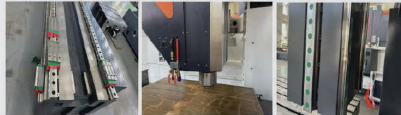
Three-linear guideway for Y-axis with door width above 2.8m
